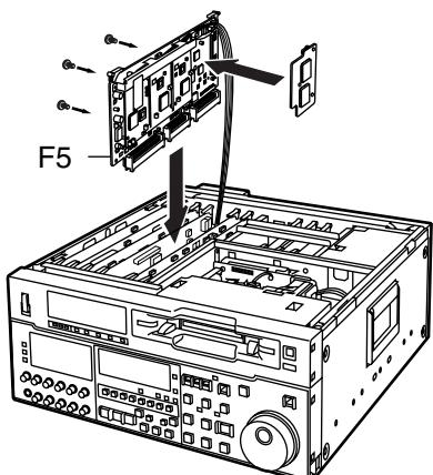
3. Install the board clamp, and attach the top panel.
