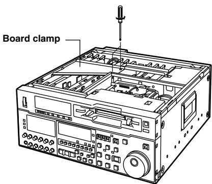
2. Attach the AJ-VNC150P board to the board in slot F5 of the main unit.
